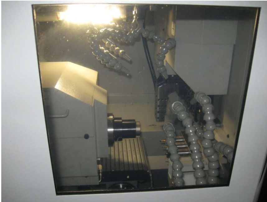
CITIZEN (Japan) A20 VII – ← Swiss Type Sliding Head 6 Axis CNC Machine
