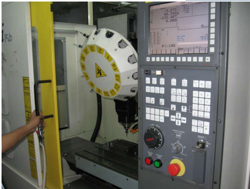
Fanuc (Japan) Drill & Tap Center (Vertical Machining Center – VMC)
